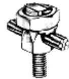
c. You may drill a hole through the side frame to accommodate a Lay-In Ground Bushing Lug such as the one shown in the illustration. Be sure to use a Lay-In Ground Bushing Lug that is rated for direct burial. Many such connectors are rated for indoor use only. You will need SS hardware – a bolt, flat washer, star washer and nut – to complete the assembly. See Figure 4 for an illustration of this assembly.
